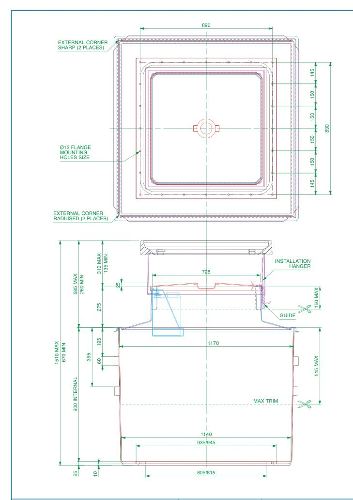
1.2m square bolted base chamber with a corbel, internal lid, adjustable skirt and square 760mm flat sealed cover. (1m square tank flange connection).
