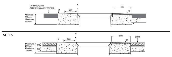
1.2m square bolted base chamber with a corbel, internal lid, adjustable skirt and square 760mm flat sealed cover. (1m square tank flange connection). For reference purposes only. This drawing is not a specification. Order against product code only. To enable continuous improvement of our products, the designs and specifications are subject to change without notice.
