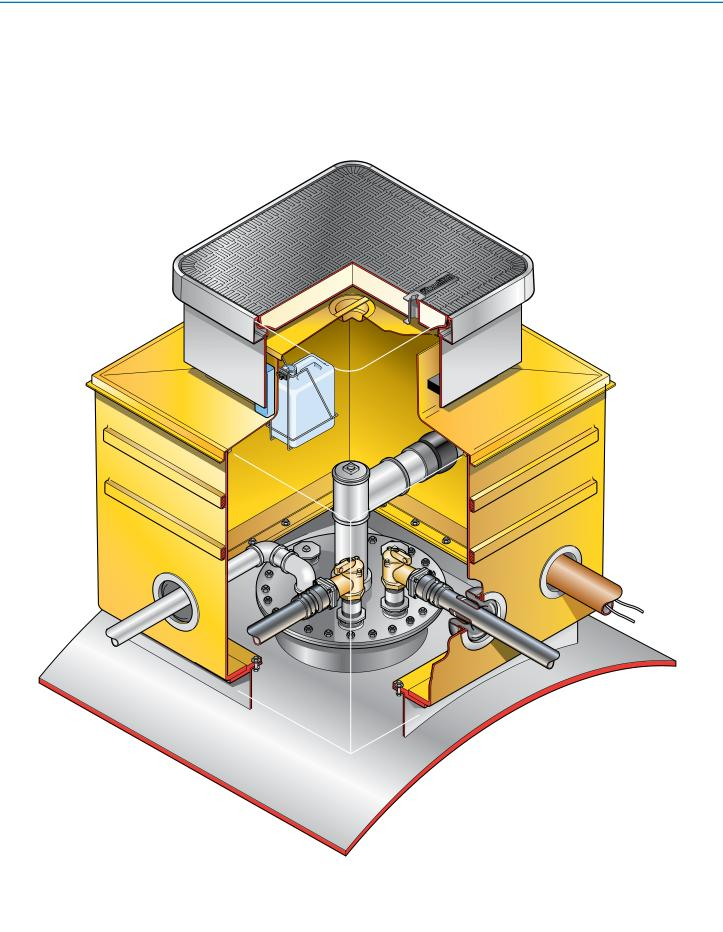
1.2m square bolted base chamber with a corbel, internal lid, adjustable skirt and square 760mm flat sealed cover. (1m square tank flange connection).
