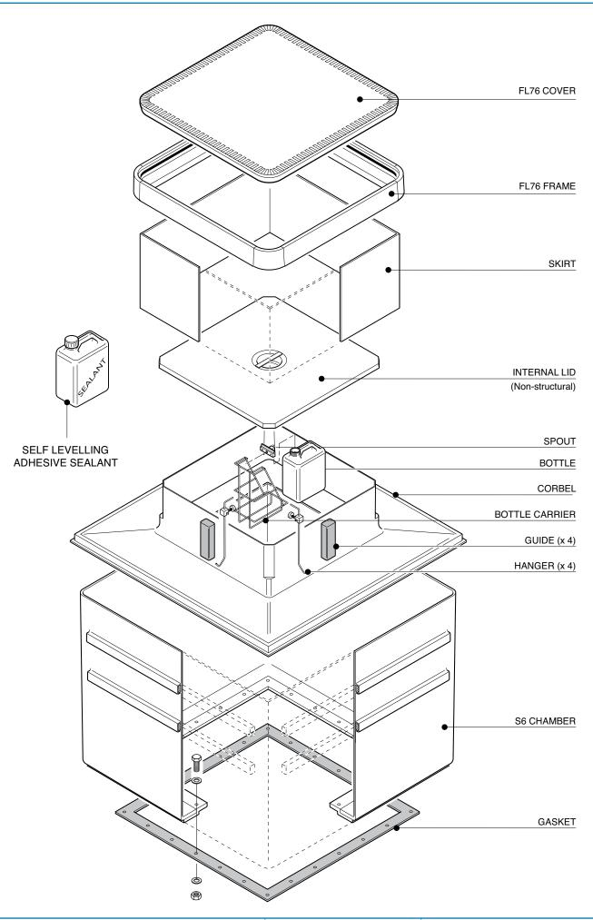
1.2m square bolted base chamber with a corbel, internal lid, adjustable skirt and square 760mm flat sealed cover. (1m square tank flange connection).
